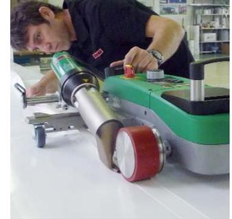
Very easy hem and piping welds with the hem- / piping welding kit
